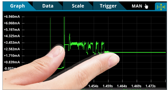
Capture the current drain from all the operating states – sleep mode to active transmit mode – of a component or a product with the DMM7510’s digitizing function. Focus in on characteristics of the wave shapes with the touchscreen pinch and zoom features.
