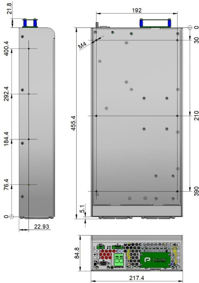
**NOTE:** All the fixing holes are M4. Maximum screw length inside the converter 5mm
